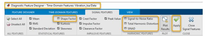
For every selected feature, the app computes a value for each ensemble member and displays the results in a histogram. Each histogram contains bins containing the number of feature values that fall within the bin range. The **Histogram** tab displays parameters that determine the content and resolution of the histograms.
