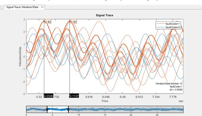
The resulting signal trace shows you that all the highest vibration peaks are associated with data from degraded systems. However, not all the degraded systems have higher peaks.
