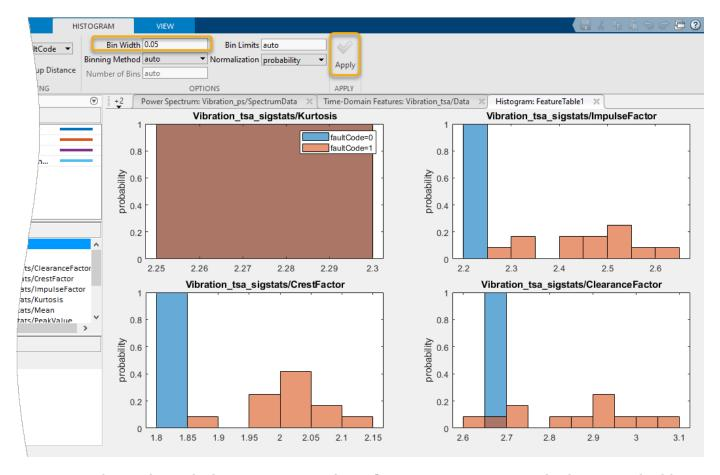
At this resolution, both CrestFactor and ImpulseFactor appear to completely separate healthy from degraded data. ClearanceFactor still has some mixed data, but to a lesser degree than with the larger bin width. Kurtosis has a smaller bin width of 0.002 with the auto bin width setting. Changing the bin width to 0.05 results in a single bin that contains all the Kurtosis data.
