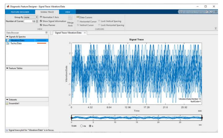
Interact with the trace plot using standard MATLAB plot tools, such as zoom and pan. Access these tools by pointing to the top right edge of the plot. You can also use the specialized options on the **Signal Trace** tab, which appears when you select the **Signal Trace** plot.
