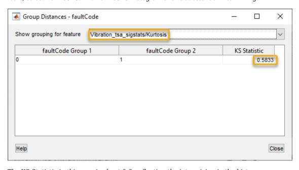
The KS Statistic in this case is about 0.6, reflecting the intermixing in the histogram.
